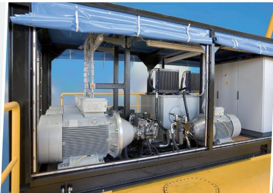
Dragflow power packs are specifically designed for use with the Dragflow Pump HY85/160 with the option of using excavators model EXHY20 or other equipments (such as winches and hoist). The power packs are based on first quality components:
