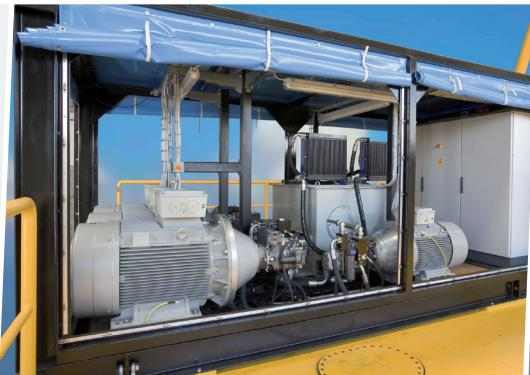
Dragflow power packs are specifically designed for use with the Dragflow Pump HY300 with the option of using excavators model EXHY35 or other equipments (such as winches and hoist). The power packs are based on first quality components:
