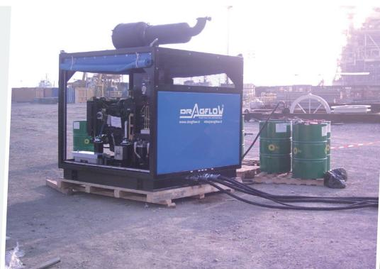
Hydraulic power pack especially designed for use with the Dragflow dredging pump models HY50/108 o HY85 with or without two excavators model EXHY20. The power packs are based on Iveco NEF N45 diesel engines, that complies with latest European emission requirements, or Electric engine.
