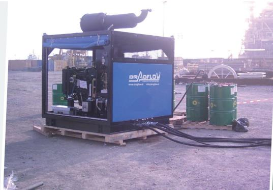
Hydraulic power pack especially designed for use with the Dragflow dredging pump models HY50 with or without two excavators model EXHY20. The power packs are based on Iveco NEF N67 or CAT C6 diesel engines, that complies with latest European emission requirements, or Electric engine.
