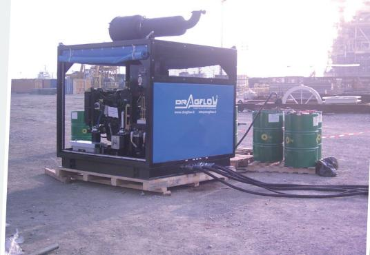
Hydraulic power pack especially designed for use with the Dragflow dredging pump models HY35B with or without two excavators model EXHY20. The power packs are based on Iveco NEF N45 or CAT C6 diesel engines, that complies with latest European emission requirements, or Electric engine.
