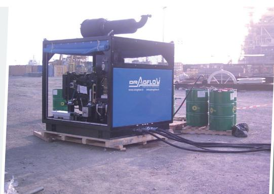
Hydraulic power pack especially designed for use with the Dragflow dredging pump models HY24. The power pack is based on diesel engine, that complies with latest European emission requirements, or Electric engine.
